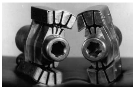
Fig 7. Feeder crusher hydraulic gear clutch with three (a) and two (b) pairs of rings
