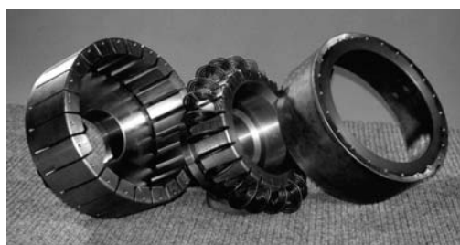
Fig 8. Composite elements of the clutch of oil pump gears
