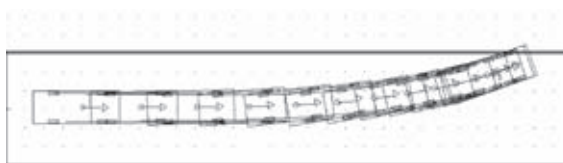
Fig 7. Movement of automobile VW PASSAT when back right wheel cannot hold up
