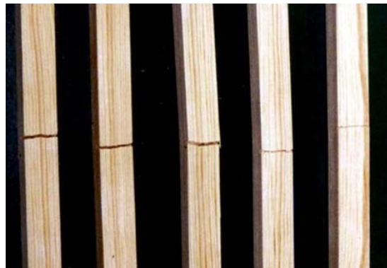
Fig 12. Smooth fractures of impregnated samples after static bending tests: a) at 230 °C; b) at 20 °C
