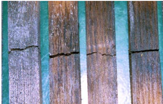
Fig 12. Smooth fractures of impregnated samples after static bending tests: a) at 230 °C; b) at 20 °C
