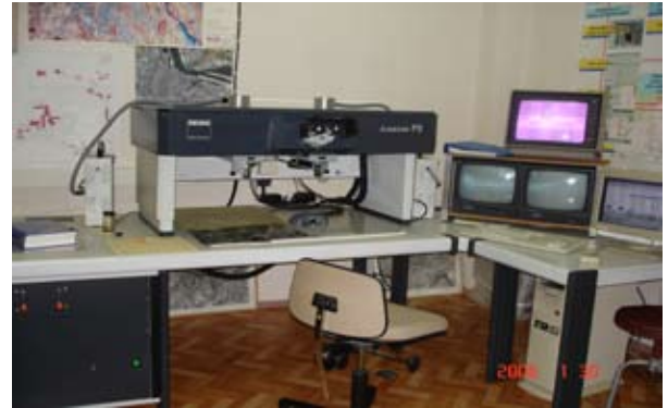
Fig 1. Analytical stereo plotter PLANICOMP P3 with a modification for education
