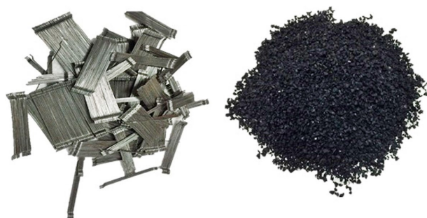
Fig. 2. Hooked end steel fiber and crumb rubber aggregate used in this study
