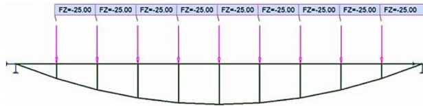
Figure 3. Load diagram when the load is transmitted through the struts
