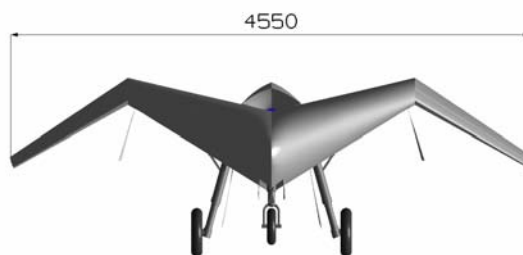
Fig 5. PW-124 – front view (span in [mm])
