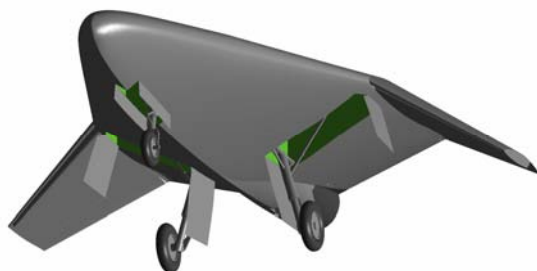
Fig 30. Internal payload containers are closed, all undercarriage legs deflected down. Double covers of each undercarriage containers are visible. Aircraft is ready to land. This is a bottom-side view
